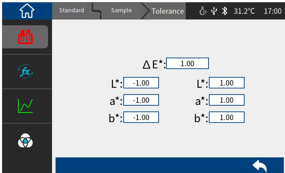
Figure 11 Standard tolerance setting interface
