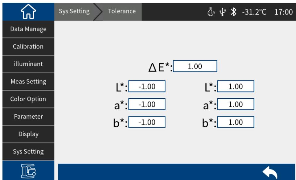
Figure 10 System tolerance setting interface
