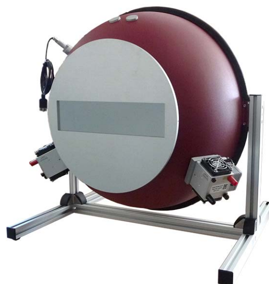
ISS Light Source with Rectangular Aperture Reducer
