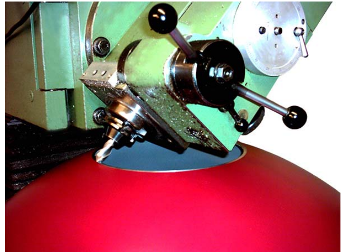
Machining of UMMP Port for use with Protection Cap
