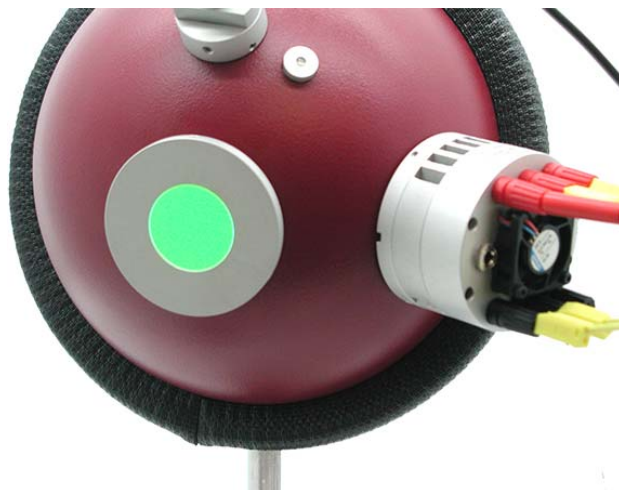
ISS-15 Integrating Sphere Source with UMPR Port Reducer mount to Standard Port Frame.
