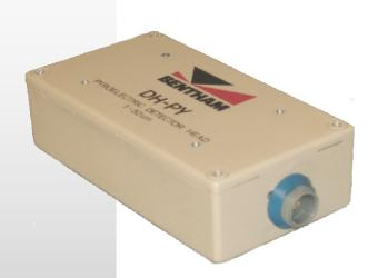
The DH-Py is a self-poling TGS pyroelectric detector, designed to operate at room temperature, which consists of window, infrared sensitive element and impedance matching amplifier.
