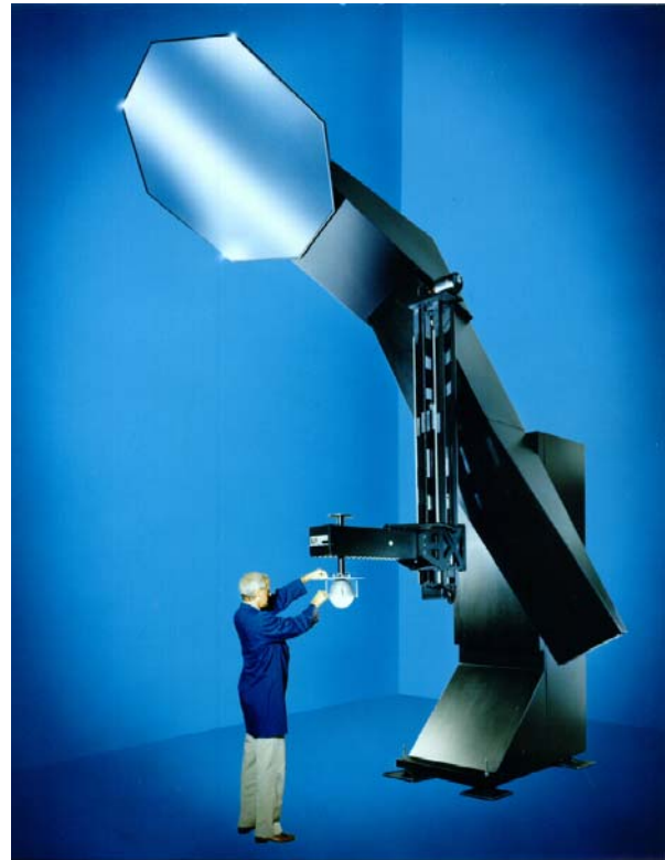
Moving Mirror Goniophotometer used to measure luminaire output, efficiency/efficacy, intensity distribution, and zonal lumen density
