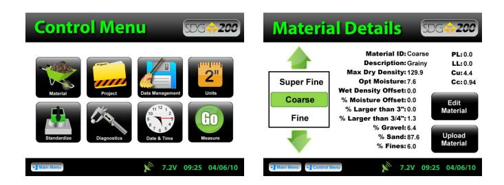
From the Control Menu, Press Material for the Material Details screen. The material highlighted in green on the left is displayed in detail on the right. To edit the details of this material, Press Edit Material.
