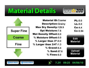
From the Main Menu, Press Start SDG 200 to get to the **Control Menu.** Press **Material** display and verify the details of the current material that will be used for this test. Once verified, Press Control Menu [1] control Monu from the status bar.
