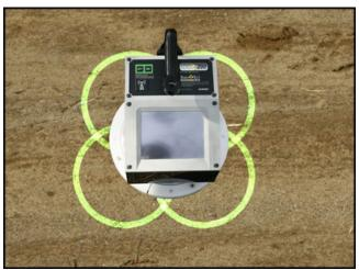
A complete test consists of five individual measurements taken in a "cloverleaf" pattern at the test location. Each of the five measurements takes about 10 seconds. The SDG 200 is placed in position 1 for the first measurement and moved clockwise around position 1 as indicated in the illustration above. Upon completion of each reading, the SDG 200 will prompt the operator to move to the next location.
