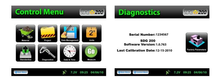
From the **Control Menu**, Press **Diagnostics** and the internal information needed for the factory to track your gauge will display. This information consists of the Serial Number, Software Version and the date the gauge was last calibrated.
