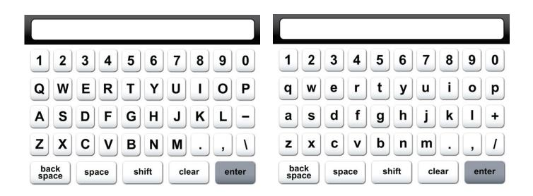
Unique yet consistent icons are located on most screens for easy one touch navigation. When data input is required of the operator the screen will display the above keyboard. Toggle from upper to lower case letters using the **Shift** button shift The upper case keyboard gives the option of a **minus sign** while the lower case keyboard gives the **plus sign** Once editing is completed simply **Press Enter** to store and return to the previous screen.
