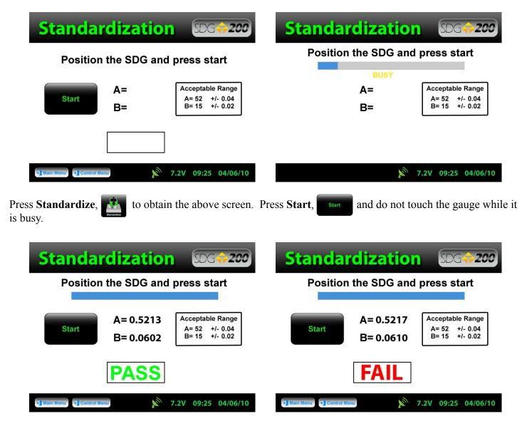
The acceptable range for the A and B values are displayed on the screen, however, the gauge will respond with a **PASS PASS** or Fail FAIL based on these ranges automatically.
