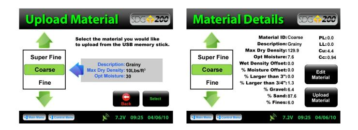
The file name of the materials located on the USB drive will appear on the left and some details identifying that specific material will be displayed on the right. Use the up or down arrows to highlight the material you wish to upload. Once verified, Press **Select** to upload the material information into the gauge. Continue to select additional materials to upload or Press **Back** to view the material in detail.
