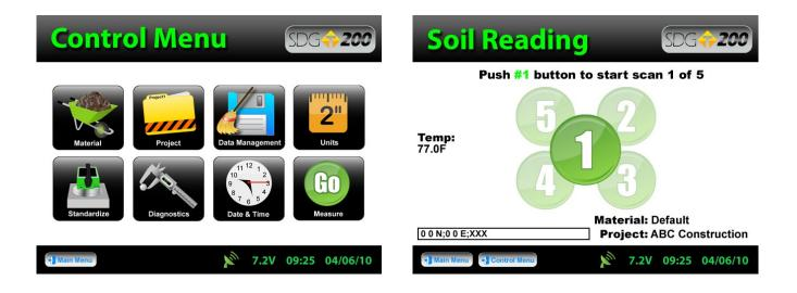
Press **Measure**, to enter into the Soil Reading screen. In the bottom left corner, the name of the material to be tested and project are displayed for verification as well as the temperature of the soil. In the bottom right corner, the GPS information is displayed. The cloverleaf pattern is also displayed for your convenience with the highlighted position being the current position to measure.
