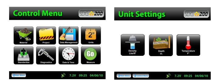
From the **Control Menu**, Press **Units.** Density, Temperature and Depth can be toggled independently between System International (SI "metric") and U.S. Customary Units. For example, you can set your Density in lb/ft³ while the Temperature is set for Celsius and Depth set to Inches. Press **Control Menu** on the taskbar to return to the Control Menu.
