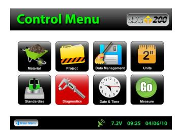
The **Diagnostic** button on the Control Menu will turn red as a reminder. Only authorized distributors or the factory are able to perform this type of calibration.
