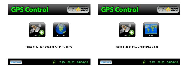
GPS formatting can also be toggled from the Universal Transverse Mercator (UTM) grid to Latitude/ Longitude (LAT-LON). Initially the display will read Sats 0 for both formats until connections have been made. The above examples show a connection to five satellites (Sats 5) in both formats. GPS locations will appear on the bottom left corner of all Reading Mode screens and will store with each reading when Data Logging is ON.
