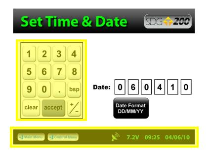
The **Status Bar** is located at the bottom of the screen (excluding the keyboard screens) and will continuously update the remaining voltage of the batteries while displaying the date, time and status of the GPS and Data Logging features.
