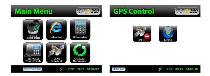
When the GPS is **ON** the satellite dish on the status bar turns from red to green.
