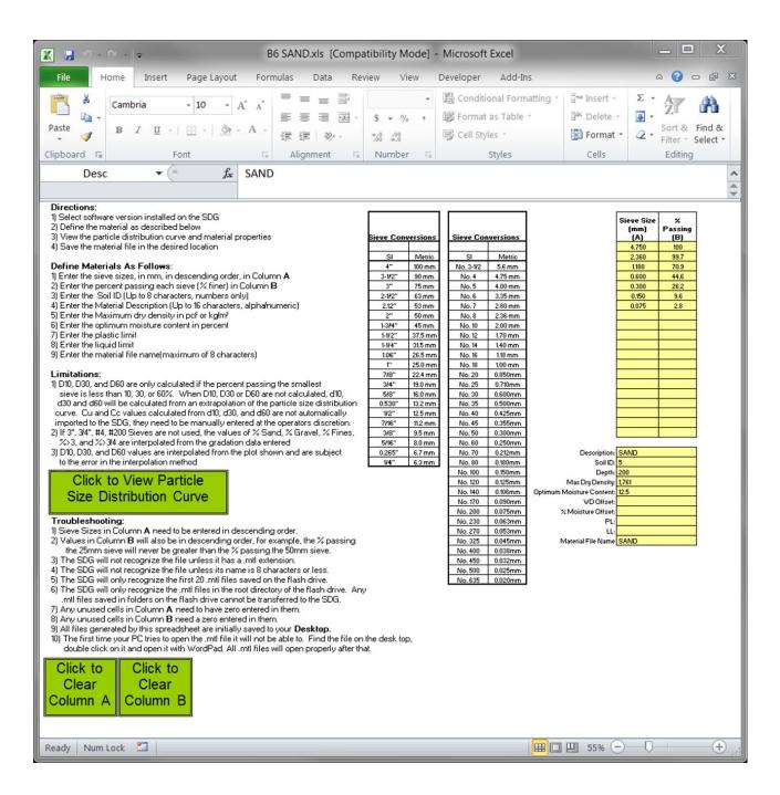
The MTL File Tool is designed to allow users to easily create .mtl files to upload into the SDG. If a gradation report completed in accordance with ASTM D 422 is available, all of the information on that report can be entered into the table on the Gradation file tool and a .mtl file will automatically be generated and saved to the Desktop of your PC. This file can then be transferred to a USB flash drive and installed directly into the SDG as explained on page 18.
