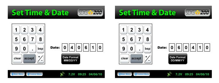
To set the date, Press **Set Date**. Set Date The date will display in either the DD/MM/YY or MM/DD/YY format which may be toggled from the button located on both screens. Pate Format As you did with the time, press the appropriate numbers for the date in the format chosen. Press Accept accept to store and return to the previous screen. (Note: Date will be preset by the factory)
