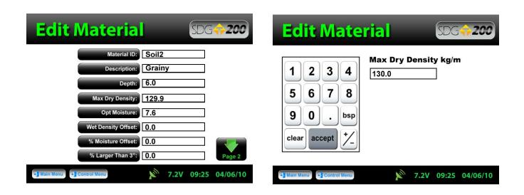
There are fifteen material properties for each material. Eight of these material properties are listed on Page one of the **Edit Material Page** and the remaining seven are listed on Page 2. Each can be edited individually by pressing its corresponding label which prompts a numeric or alpha numeric keypad.
