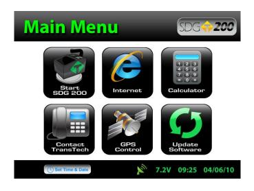
Turn the SDG 200 on by pressing the ON button. After a few seconds the TransTech splash screen will appear followed by the Main Menu Screen. The Main Menu screen will display six options. Start SDG200, Internet (Coming Soon), Calculator, Contact TransTech, GPS Control and Update
