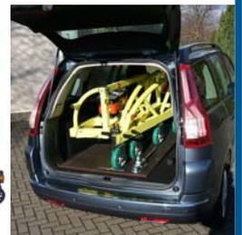
The planograph AX<sup>®</sup> 02 is characterized by a high-quality aluminium and stainless steel construction.
