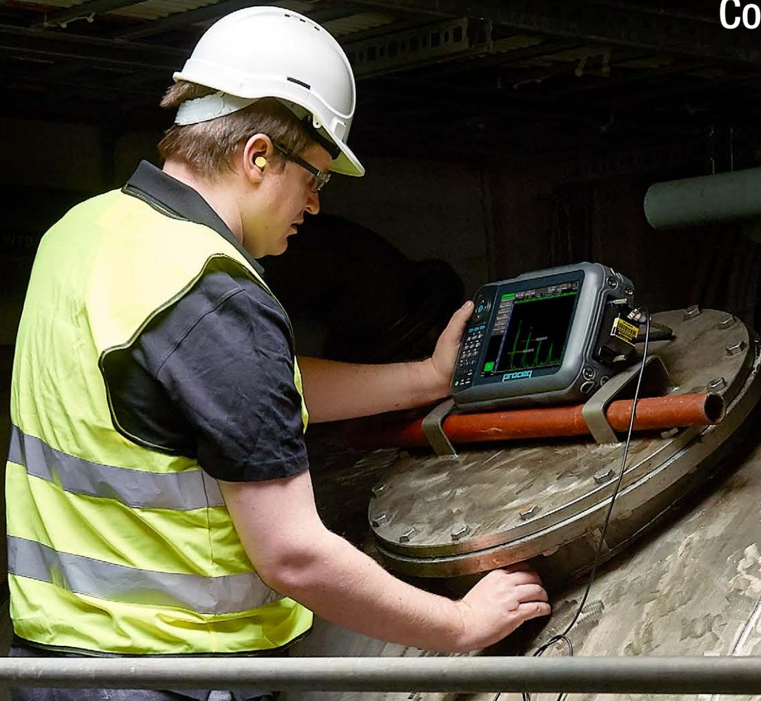
A, B and C scan data displays with a choice of multiple layouts enable a broad range of inspection applications:
