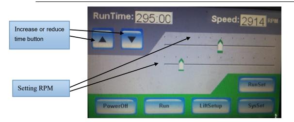
4.2.5 Enter Runset menu to quickly set up the time and RPM
